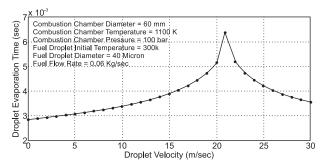
Figure 7: Effects of droplet velocity on required evaporation time.
