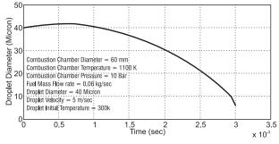
Figure 3: Fuel droplet diameter in heating phase.
