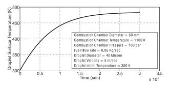
Figure 4: Fuel droplet surface temperature in heating phase.
