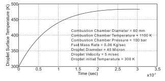
Figure 6: Fuel droplet surface temperature for its complete life time.
