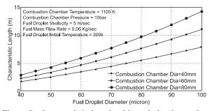
Figure 9: characteristic length with variation in combustion chamber diameter.
