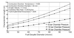
Figure 8: chamber pressure effects on characteristic length.
