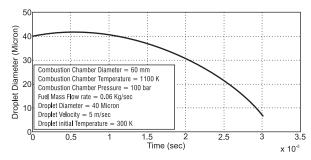
Figure 5: Fuel droplet diameter with time.
