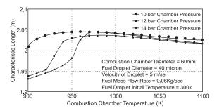
Figure 11: Unusual behavior of characteristic length against chamber pressure and temperature.
