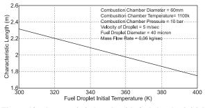
Figure 13: characteristic length with fuel droplet initial temperature.
